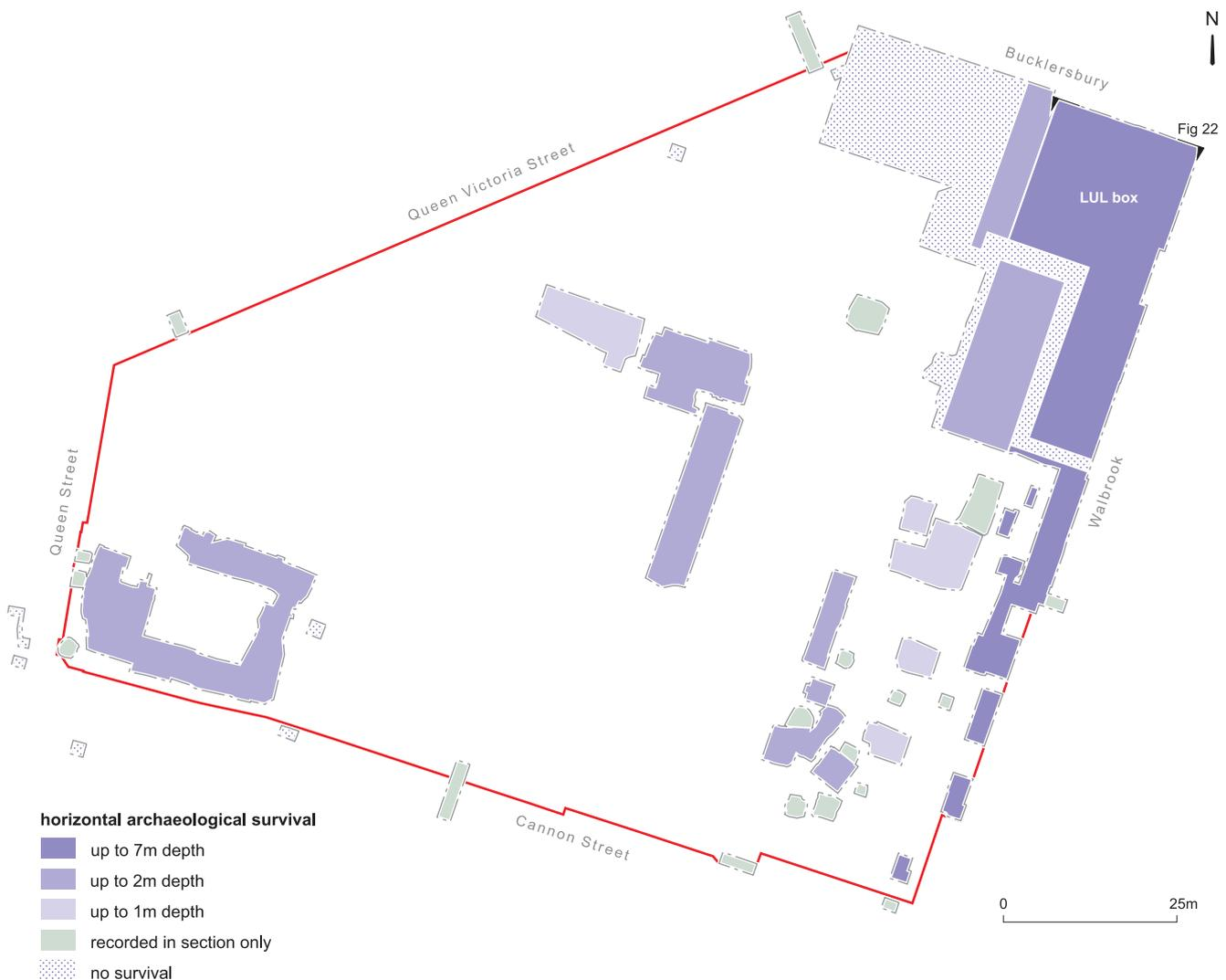
Fig 2 Plan of the areas of archaeological excavation undertaken under site codes BBU05 and BZY10; the toning in the excavated areas represents the varying levels of archaeological survival due to previous truncation (scale 1:1000)
