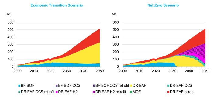
Source: BloombergNEF. Note: BF-BOF – Blast furnace basic oxygen furnace route, DR-EAF – Direct reduction electric arc furnace, CCS – Carbon capture and storage, H2 – Hydrogen, MOE – Molten oxide electrolysis.
