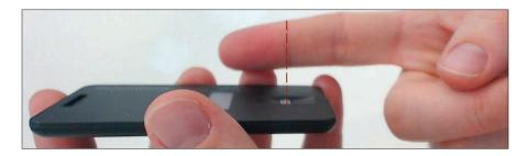
• Make sure your finger is straight along the center of the B-Unit 3 and that you swipe in a straight line downward over the sensor.
