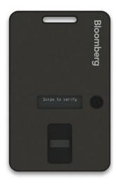
• Hold the B-Unit 3 up to the flashing area on the screen, lining up the B-Unit 3 device with the on-screen graphic. If the B-Unit 3 displays shows 'Move closer to the monitor' you may need to move the B-Unit 3 closer to the monitor or make sure the B-Unit 3 is aligned to the B-Unit 3 on-screen graphic. The B-Unit 3 display will show a progress bar indicating that data is being received.
