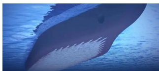
Figure 16: Illustration of Silverstream’s air lubrication system beneath a vessel
